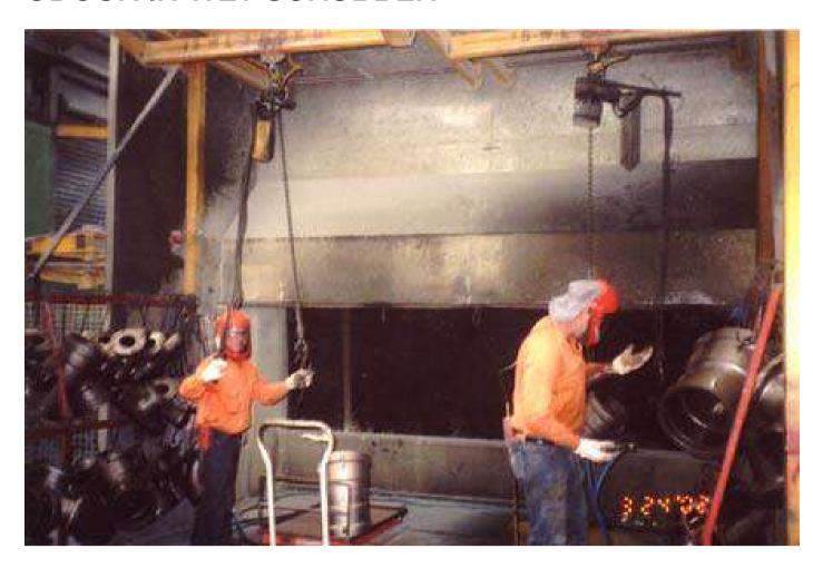
The pictured spray booth is used for solvent and water-based paint primers and is fitted with a wet scrubber, using **Triple7 Odour Control.**
