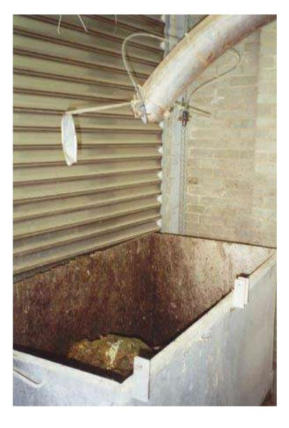
Untreated sewer from initial stage of treatment. **Triple7 Odour Control** is misted over bin by nozzles attached to outlet pipe.
