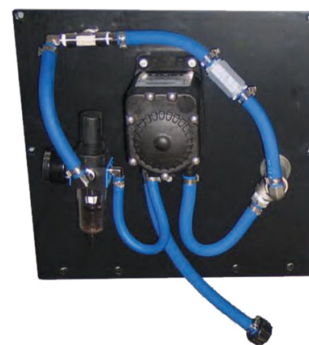
FloJet Pump Configuration
