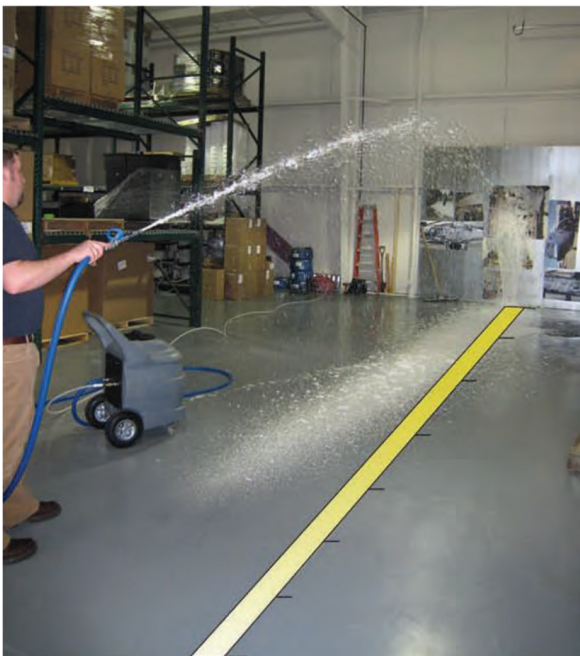
Horizontal Throw with FloJet Pump (11 Meters)
