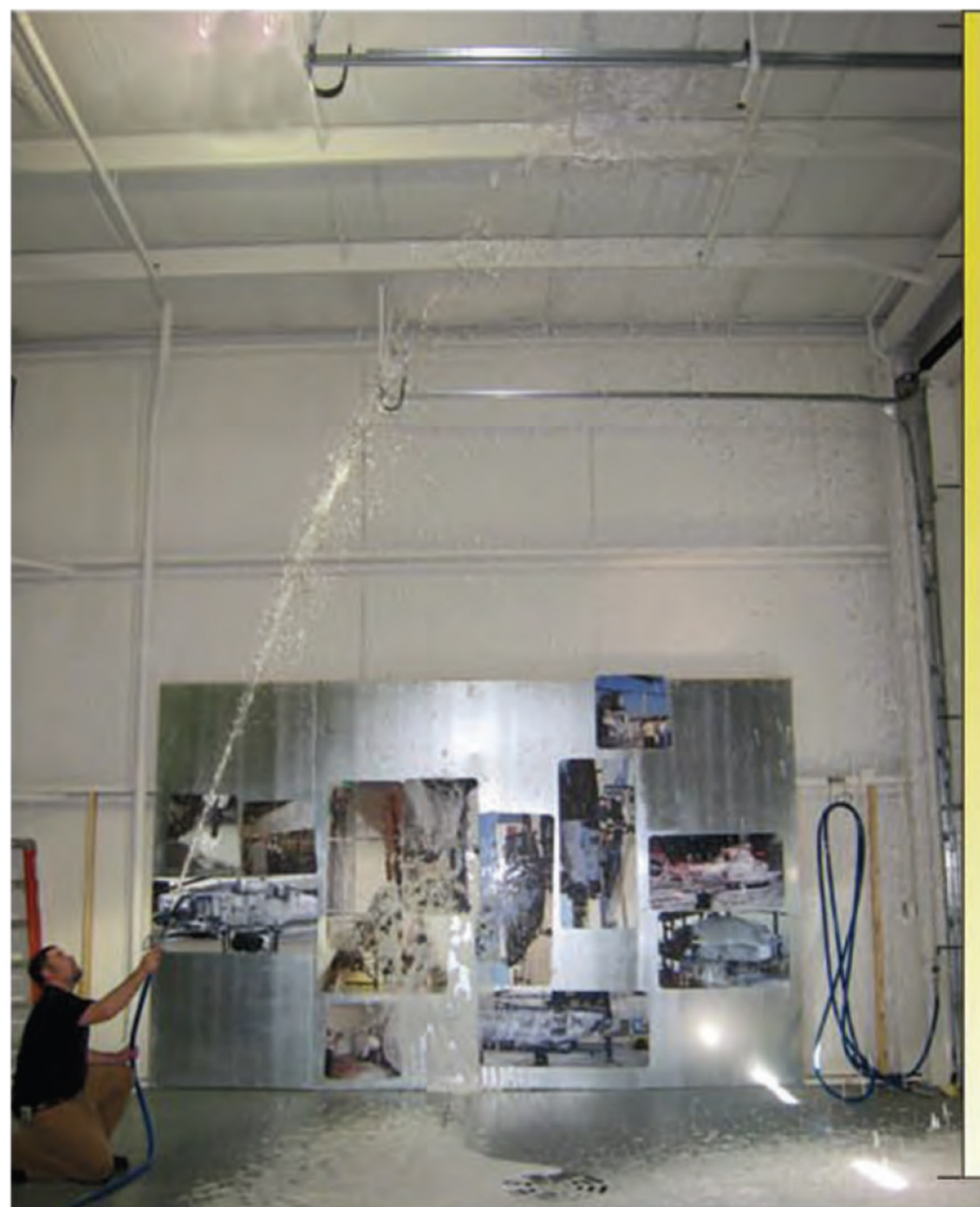
Vertical Throw with FloJet Pump (8 Meters)
